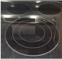
**Electric glass ceramic** range tops have electric resistance heating elements located under a sealed, ceramic surface. The element radiates heat through the glass ceramic surface and subsequently heats the bottom of the pan. The temperature under the glass ceramic surface is significantly higher than the temperature of the pot. Because the ceramic/glass construction is subject to cracking at higher heats, a temperature limiting control is used to prevent failure.
