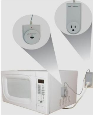
The Safe-T-sensor, developed by Pioneering is the only technology of its kind that helps mitigate the many fires and false alarms attributed to the use of microwave ovens. The Safe-T-sensor is a patent pending technology designed to detect burning conditions within the microwave and to shut the microwave off before it causes a fire or triggers the fire alarm.
